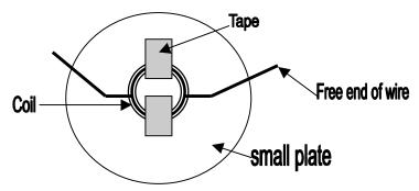
4. Pass out two disk permanent magnets. Have the families place one magnet in the center of the coil and the other magnet in the same spot but on the other side of the plate. Now if one permanent magnet moves so will the other and the plate will be forced to move as well.
